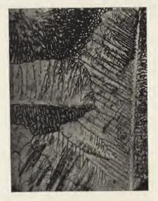
Fig. 13. (x 30 Diameters. Vertical Illumination.) Dendritic Structure of Tin Cast on Stone.
